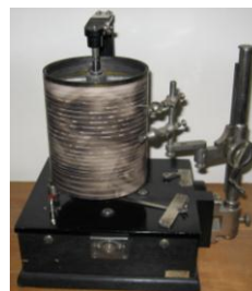
Figure 7: Kymograph used for intonation research and below a sample made by the device.
