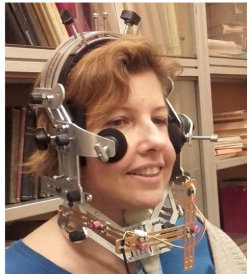
Figure 1: Ultrasound stabilization helmet with the fixed ultrasound transducer and lip camera (in the front of the lips)
